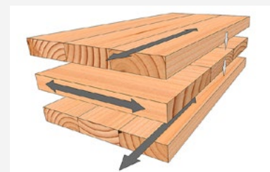
CLT, Cross-Laminated Timber, consists of solid wood panels built up by gluing together layer upon layer of planed and strength-graded boards of timber from environmentally certified Swedish forests.
